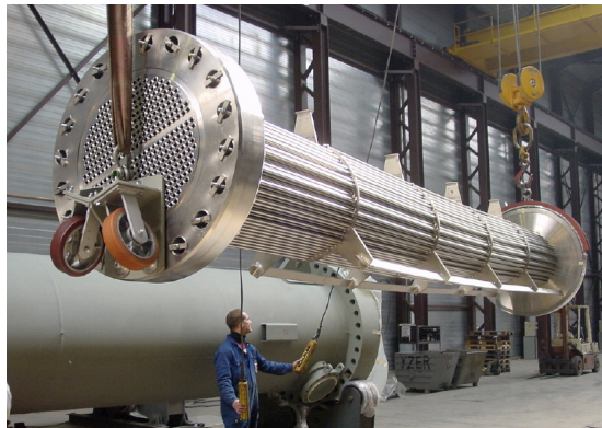
Left to right: POX Autoclave, PTA Heat Exchanger
